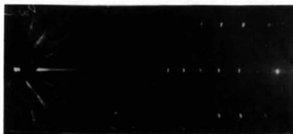
Fig. 2. a -axis 15^\circ -oscillation photograph of a melt-grown Pb-doped crystal, showing reflections of the most common polytype 4H . 3 cm camera; \text{Cu K}\alpha radiation.
